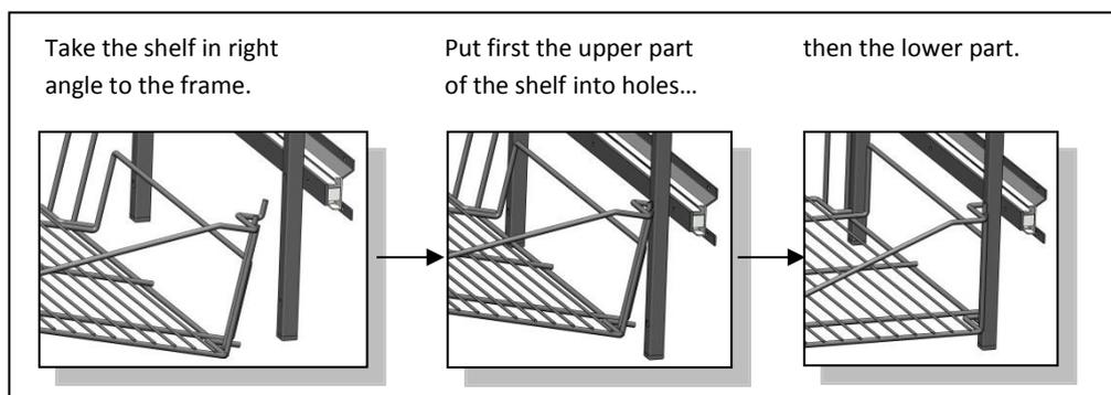
Picture 2 – fixing the frame
